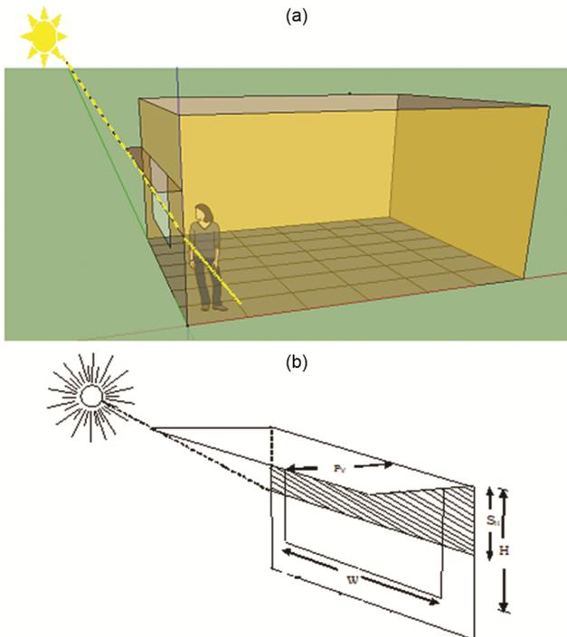
Fig. 3a) — Schematic diagram of overhang shading a) 3D representation of schematic of shading and direct solar radiation interaction, b) Schematic for projection of overhang shading on the fenestration
