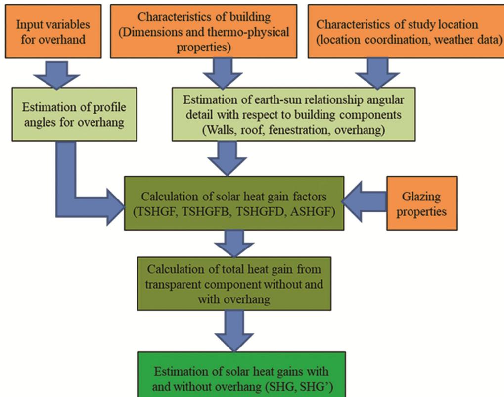
Fig. 1 — Flow diagram of the complete process used in this study
