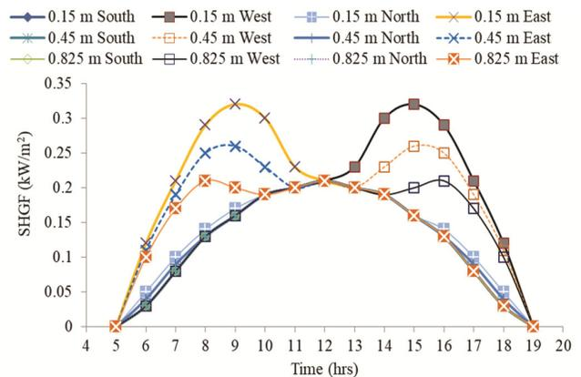
Fig. 6 — Effect of overhang width on the SHGF in the month of June
